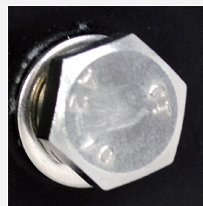
Use 304 stainless steel screws
