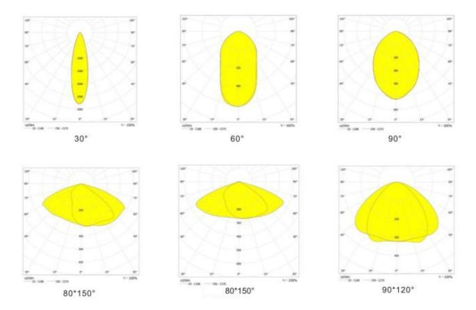
Note: LED optical rotation performance of different color temperature is deviated, the deviation value is  $\leq$  5%. The light source test data is based on Philips Luxeon LED 5500K.
