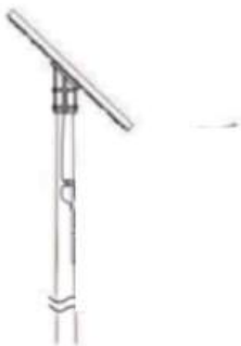
3. Connect the panel bracket with the bracket, and connect the solar panel. The front is installed facing south (the northern hemisphere is installed facing south, installed in the southern hemisphere to the north).
