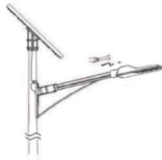
4. Connect the cable in the lamp holder with the cable of the battery panel and battery box. Connection (the cable passes through the bracket tube and is connected with the corresponding joint), Finally, fasten the lamp holder on the bracket.
