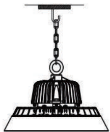
2. Hanging chain installation method
